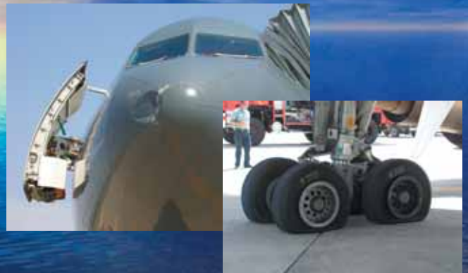
Airbus 310 bird strike at LDZA during take off run - only one tire left after immediate braking
