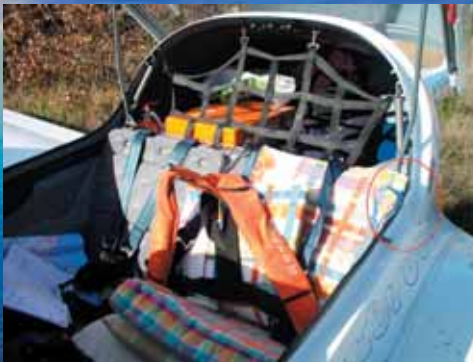
DA-20 canopy unlocks and open mid-flight: seat cushion jammed in canopy frame
