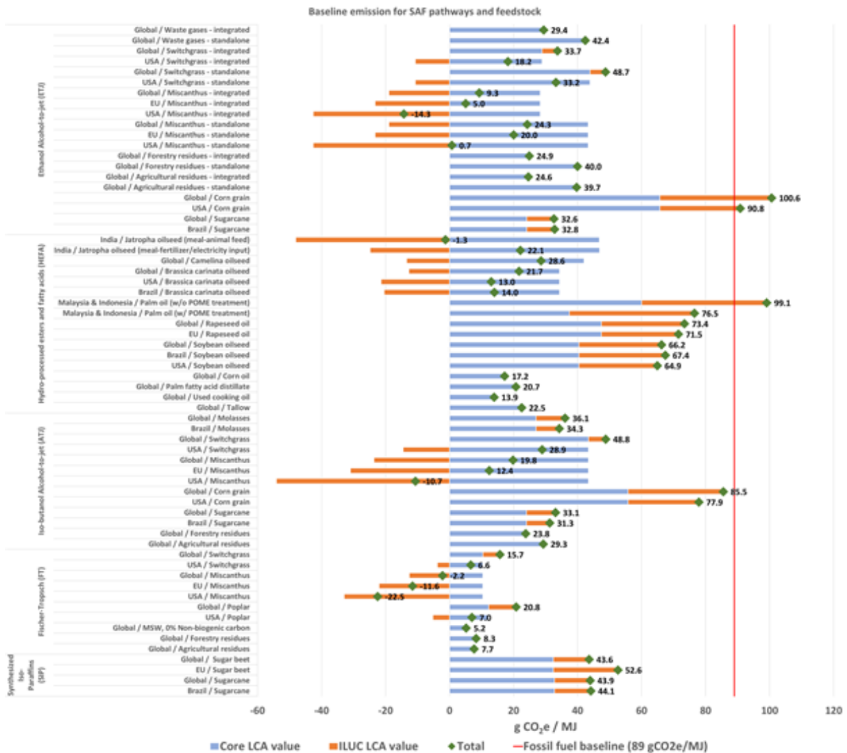
Figure 10 LCA emissions for CORSIA eligible SAF pathways and feedstock compared to CORSIA fossil fuel reference value (89 g CO 2 e/MJ) [19]27
